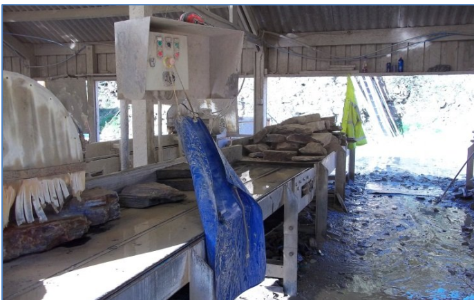
Plate PP/7: Saw benches showing stone to be cut.
